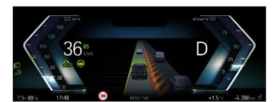
As part of Assisted Driving Mode, the emergency lane assistant makes it easier to form an emergency lane as required by law in many countries. This means that the vehicle automatically positions itself on the right or left side of the road in a traffic jam situation, depending on the lane being driven in. Available in the following countries: Germany, Austria, Luxembourg, Switzerland, Slovenia, Hungary, Czech Republic, Poland, Slovakia and Belgium.
