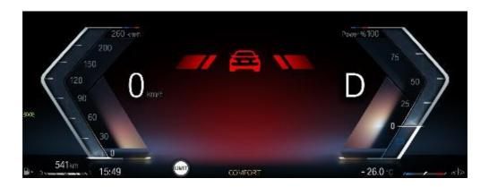
Front collision mitigation with brake intervention helps prevent collisions. The system can detect oncoming vehicles. In an emergency, the system can prevent a collision or significantly reduce the impact speed.
