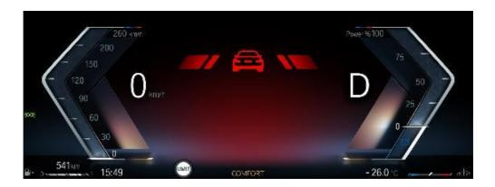
If the front collision mitigation clearly detects the end of a traffic jam, the system can bring forward the intervention time of the brake intervention and, in an emergency, ensure a significant reduction in the impact speed.
