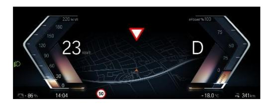
In addition to the right-of-way signs "Observe right-of-way" and "Stop" signs, your right-of-way warning now supports you at traffic lights.
