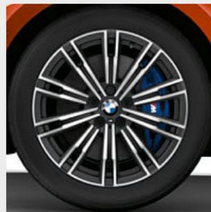
■ 18" M light alloy Double-spoke style 790 M wheels, Bicolour Orbit Grey, front 7.5 J x 18 with 225/45 R18, rear 8.5 J x 18 with 255/40 R18 run-flat tyres. Standard on M Sport models.<sup>1</sup>
