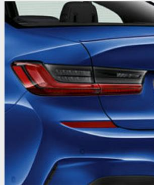
■ The rear lights with their characteristic L-shape and lighting elements in full LED technology identify the vehicle as a BMW even in the dark.
