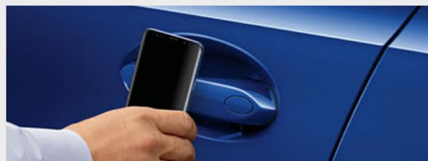
□ Comfort Access enables keyless access to the vehicle through all doors and the tailgate. It also includes a Digital key for locking and unlocking as well as starting the vehicle using a compatible smartphone<sup>3</sup>. Only available as part of the Comfort package.
