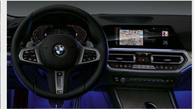
■ The BMW Live Cockpit Professional features a display cluster consisting of a fully digital 12.3" instrument display and a high-resolution 10.25" Control Display as well as the BMW Operating System 7.0. Exclusively available as standard for M Sport, M Sport Plus Edition and M340i xDrive models.
