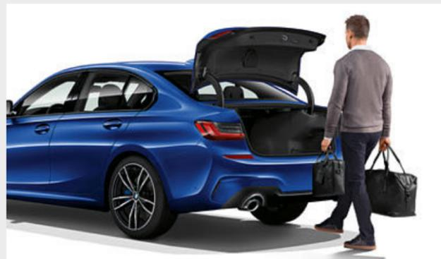
□ Automatic tailgate operation allows remote opening with a key and closing of the tailgate by simply pressing the tailgate button or key. The tailgate can also be opened in the conventional manner, using the outside handle, and closed pressing a button on the inside of the tailgate. Only available as part of the Comfort package.
