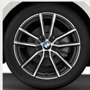
■ 18" light alloy V-spoke style 780 wheels, Bicolour Orbit Grey, 7.5 J x 18 with 225/45 R18 run-flat tyres. Standard on Sport models.<sup>1</sup>
