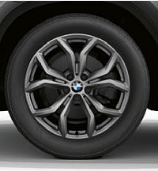
■ 19" light alloy Y-spoke style 694 wheels, Ferric Grey with run-flat tyres, wheel size 7.5J x 19 with 245/50 R19 tyres.
